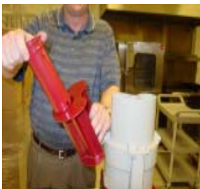
Step 8: Place Long Pusher in round slot of Pusher Assembly.
