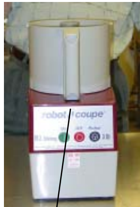
Step 2: Rotate bowl counter clockwise until handle is centered in front.
